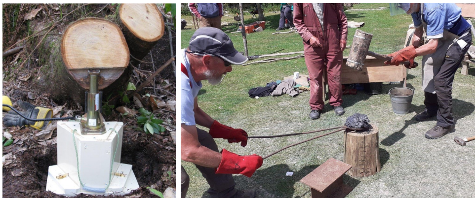
(Left) compressing the pre-fabricated clay blocks in a mould using a car jack, and (right) consolidating one of two parts of the bloom
