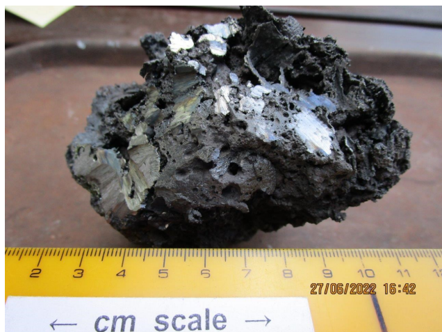
Iron content of bloom revealed on cutting
